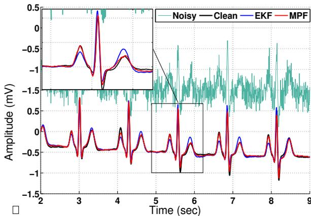
Fig. 2. Typical filtering results of EKF proposed in [4] and MPF with 2000 particles for a noisy ECG signal of 0dB. On the top: input signal; on the bottom: original clean signal (dark green), EKF filtered output (blue) and MPF filtered output (red).
