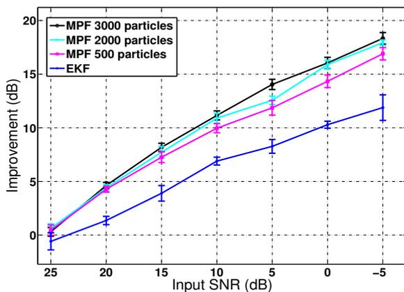
Fig. 3. MPF with 3000, 2000, and 500 particles and EKF filter output SNR improvement versus different input SNRs for 20 portions selected from the MIT-BIH Normal Sinus Rhythm database, averaged over 20 Monte Carlo simulations each.
